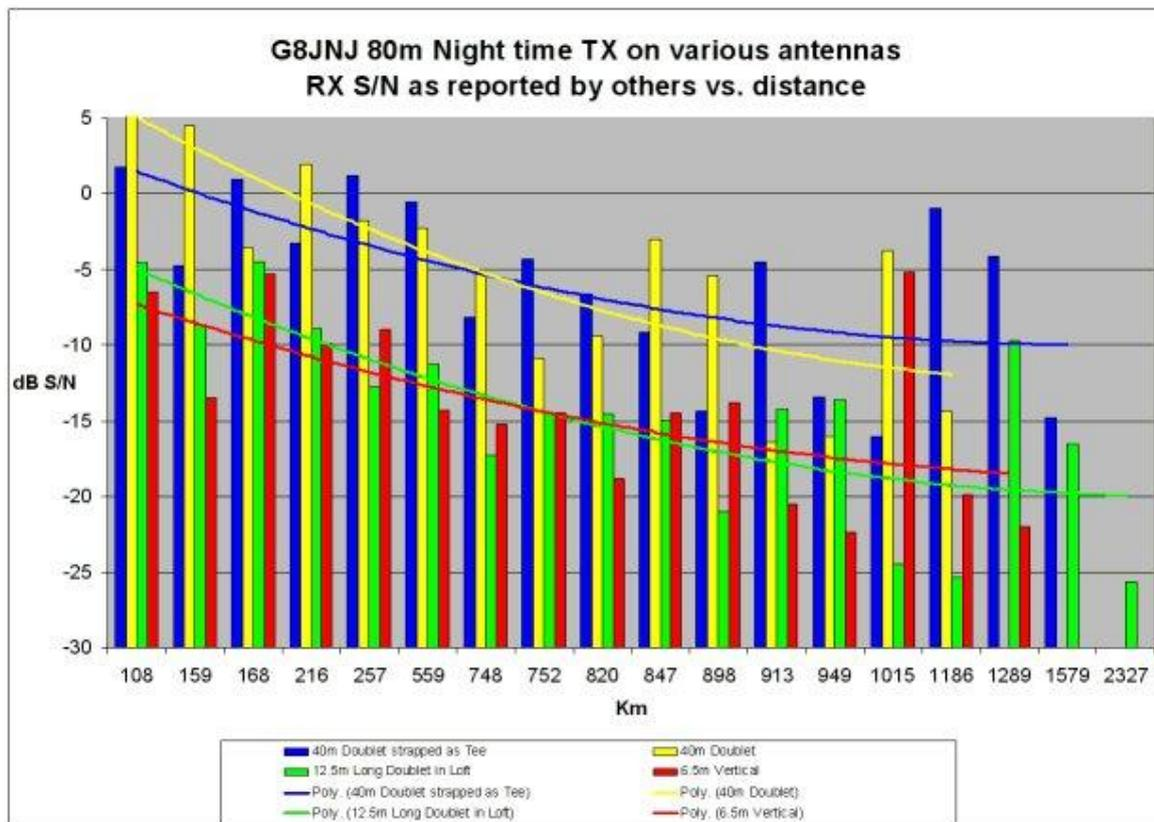
I've improved upon the accuracy of distances between stations this time, as the previous 160m plots used the same distance references for all the sites. This time I've plotted the correct distances between stations.
