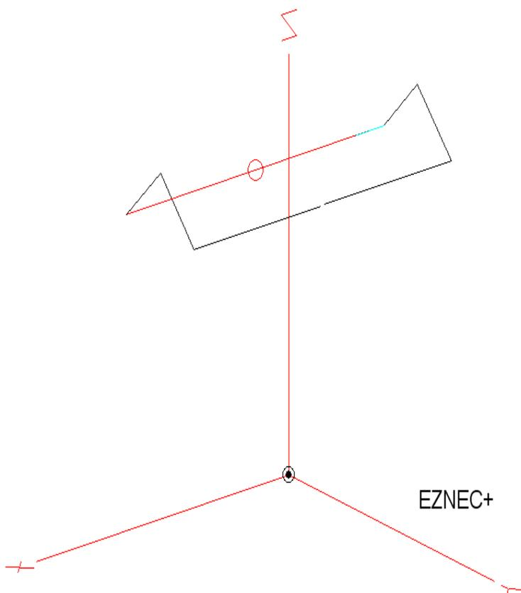
This was very disappointing. The although it provided a slightly more Omni-directional pattern on the HF bands. The gain was noticeably lower (10dB worse on 80m) in comparison to the previous Zigzag dipole, so it was quickly abandoned. In theory this antenna should have worked much better than it did, I think part of the problem was the close proximity of the wire elements to the structure of the building and the mains wiring.
