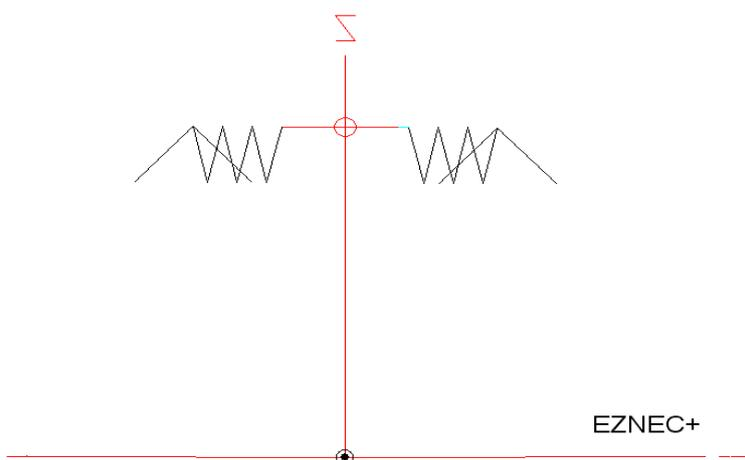
This lowered the resonant frequency which improved the performance on 80m slightly; however it still proved a difficult match on some of the HF bands, where it was approaching  $\frac{1}{2}$  wave long.
