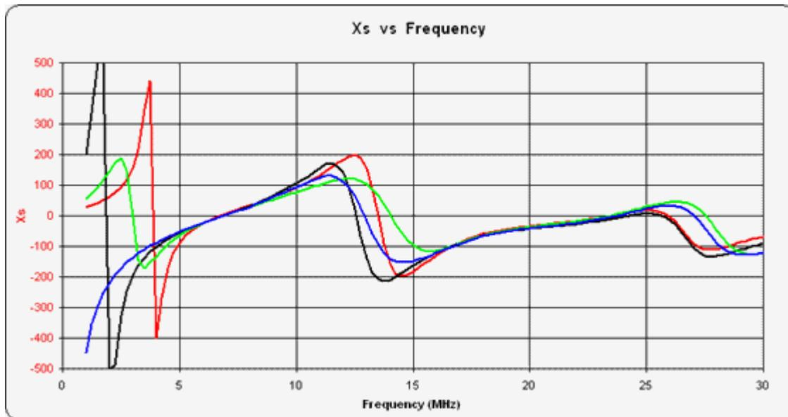
So at frequencies where the 33ft radiator presents a high feed impedance (14 MHz and 28MHz) the very rapid change in Reactive impedance causes an observable difference between the curves. The FT40-61 and T200A-2 cores have practically the same values, and as expected the lossier Ferrite and Iron powder cores present a slightly lower impedance, except at 28MHz.
