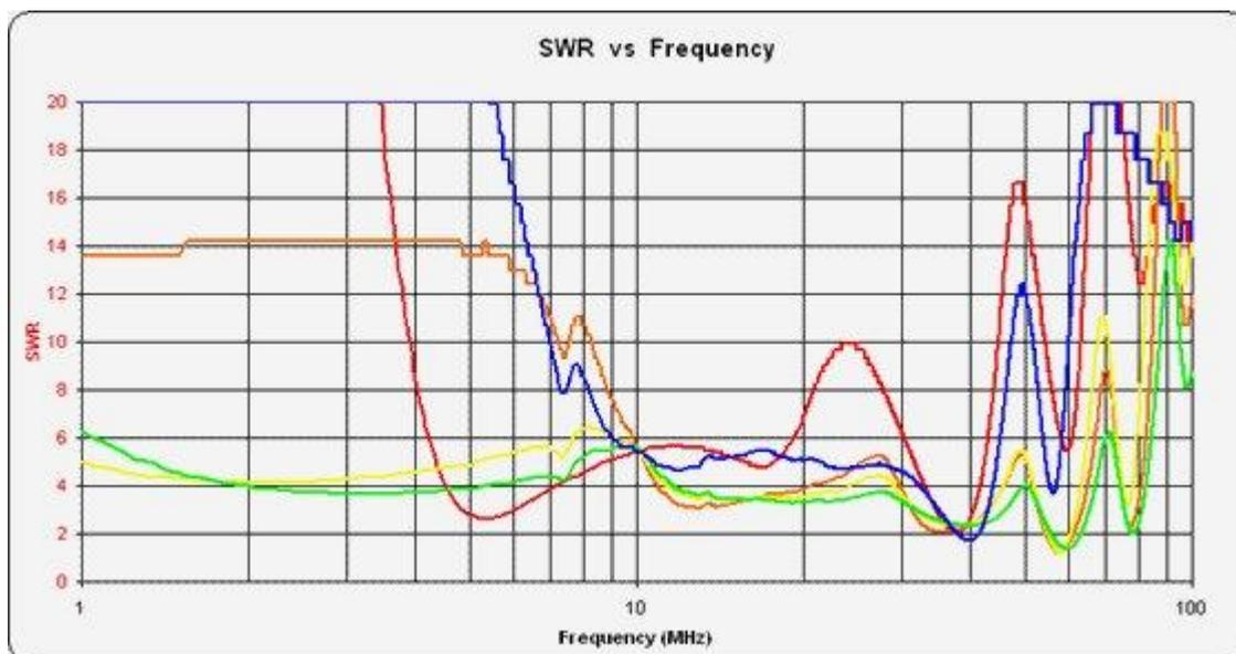
When required, I use a 4:1 Unun which I have specially optimised for this application, it is lossy but the improvement in match to 50 ohms offsets the mismatch loss which would otherwise occur along
