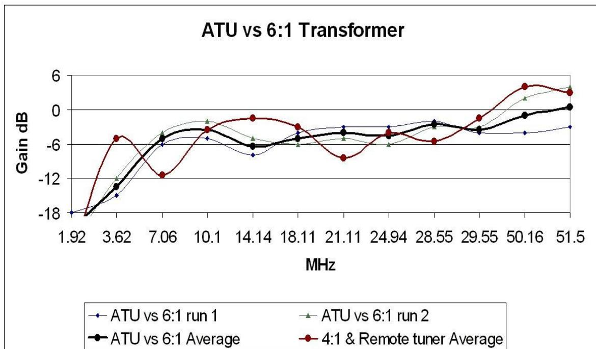
It shows field strength measurements I made some time ago, which compare a 30ft vertical fed with an auto-tuner at the base vs. the same antenna fed a 4:1 balun wound with 75 ohm coax on two separate type 43 ferrite cores and a remotely sited tuner fed via 200ft of low loss LDF2-50 coax vs. a broadband antenna of the same element length.
