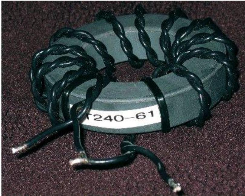
This gave good performance from 1.8 to 52MHz, with less than 0.1dB loss over most of the range up to 30MHz, and approx. 0.5dB at 50MHz. This was measured with a miniVNA by halving the loss of two Ununs connected back to back I could have added more turns without affecting the performance over 1.8 to 30MHz (I started at about 15 turns) but I found could achieve sufficient bandwidth to include 50MHz by sacrificing a bit of additional loss at each end of the operating range.
