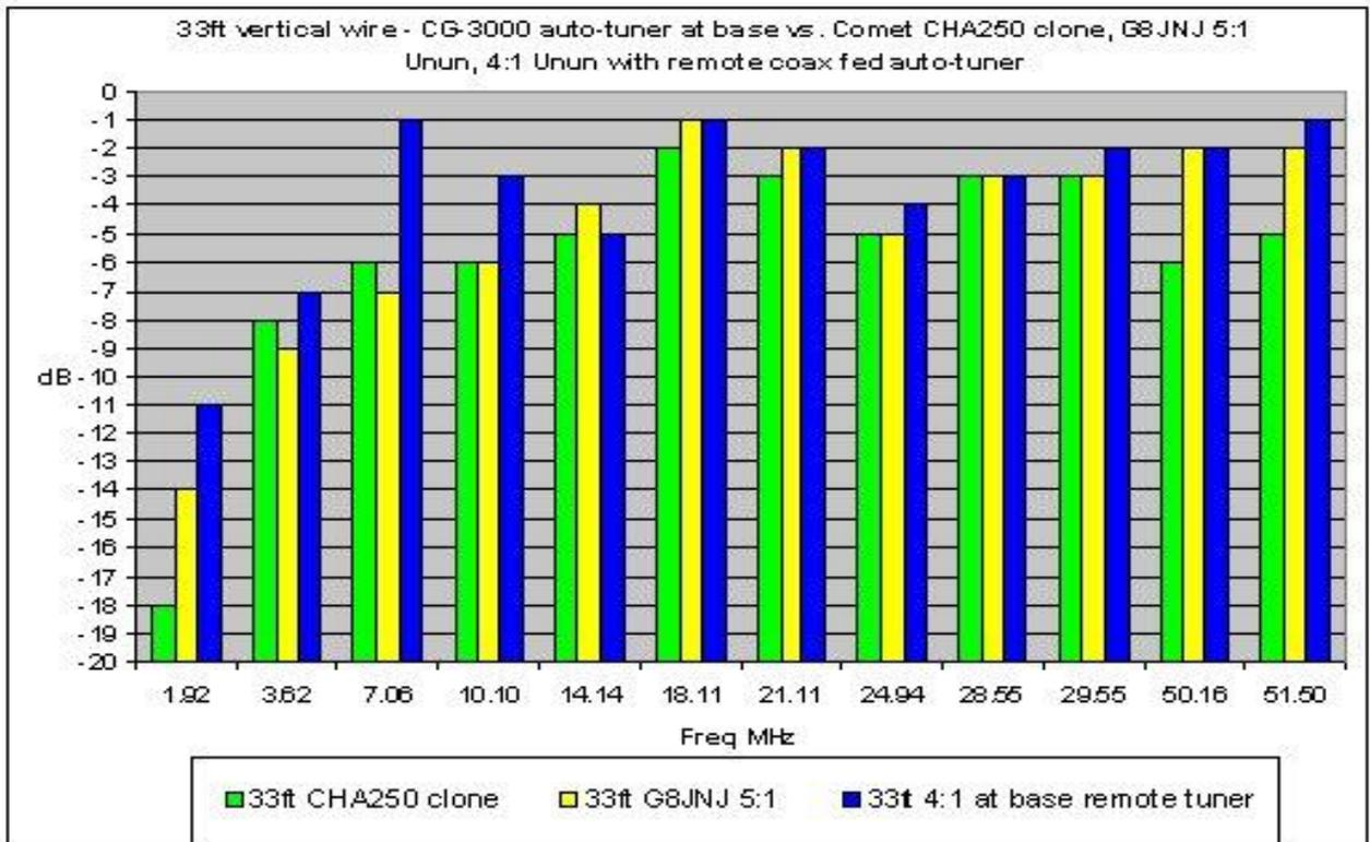
Note that both the Comet copy and G8JNJ Ununs were used without any tuner attached. They both rely upon losses in the Unun to provide a good match to the TX.
